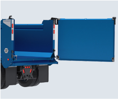
Swing / Barn Door Manually swing tailgate out of the way and attach to side of body for dumping
